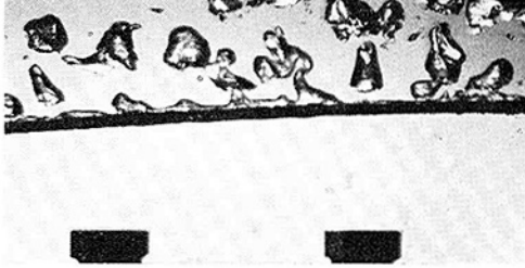
Fig. 3(f) g = 26g_c, R = 0.0200 in., acetone, q = 60,000 \frac{\text{Btu}}{\text{ft}^2\text{hr}}, R' = 1.64
